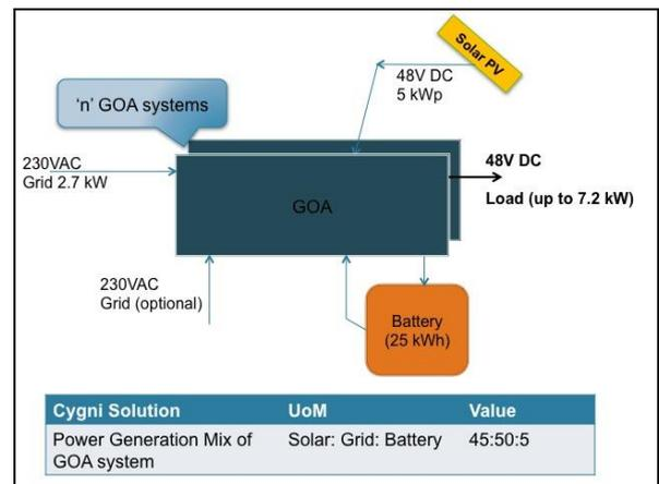
Figure 2: GOA System Block Diagram
